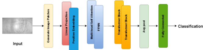
Fig. 6: Architecture of VisionTransformer model.
