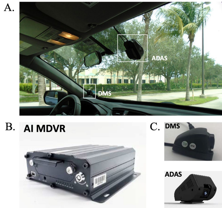
Fig. 2 A Installation of AI (Artificial intelligence)-embedded cameras. The Advanced Driver Assistance System (ADAS) camera faces outwards and is located at the top center of the windshield. The Driver Monitoring System (DMS) faces the participant driver and is located at the bottom left of the windshield. B Close-up of the Artificial Intelligence Module Digital Video Recorder (MDVR). C The ADAS and the DMS
